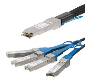
The QSFP4SFPPC1M is an MSA Compliant QSFP+ direct-attach Twinax breakout cable. It is designed, programmed and tested to bridge 40G network equipment with 10G compatible servers or routers. This passive Twin axial cable connects a single QSFP+ port to four 10G SFP+ ports and is fully hot-pluggable making upgrades and replacements seamless by minimizing network disruptions.
